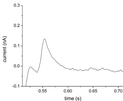
**Figure 2.** Measurement of a transient current resulting from a 50 mM  $\text{Na}^+$  concentration jump on the empty SSM membrane. The solutions are switched at 0.5 s from NA (containing no  $\text{Na}^+$ ) to A (containing 50 mM  $\text{Na}^+$ ). The initial trace before  $\sim 0.55$  s results from the switching of the valve. The transient current response is positive and has a pictured maximum of  $\sim 0.09$  nA.
