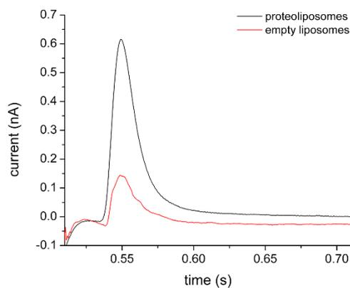
**Figure 3.** Measurement of a transient current resulting from a 50 mM  $\text{Na}^+$  concentration jump on PaNhaP proteoliposomes (black trace) or empty liposomes (red trace). The solutions are switched at 0.5 s from NA (containing no  $\text{Na}^+$ ) to A (containing 50 mM  $\text{Na}^+$ ). The initial signal before  $\sim 0.55$  s results from the switching of the valve. The transient current response was positive for proteoliposomes and had a maximum of  $\sim 0.6$  nA.
